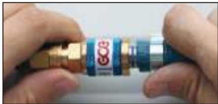
3. Mounting is finished. O-ring is visible.
