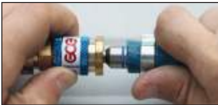
2. Pull the "blue" sleeve of the Quick connector and insert the coupling pin into the Quick connector.
