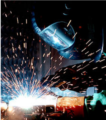
Gas metal arc welding
