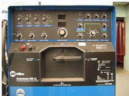
A high output [welding power supply](#) for SMAW and [GTAW](#)
