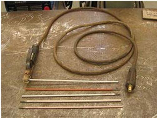
Various welding electrodes and an electrode holder
