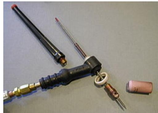
GTAW torch, disassembled
